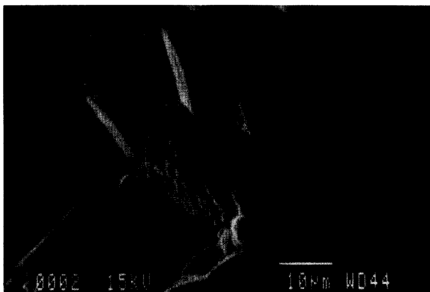
Fig. 2. Secondary electron image micrograph showing deposition of euhedral calcium carbonate crystals about 10 to 15 \mu\text{m} long on the bar's surface.
